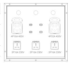
Every socket include circuit breaker. Power Output protected by Earth Leakage Relay.
