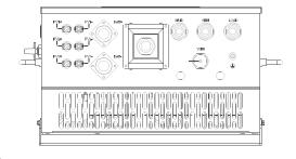
Every socket include circuit breaker. Power Output protected by Earth Leakage Relay.
